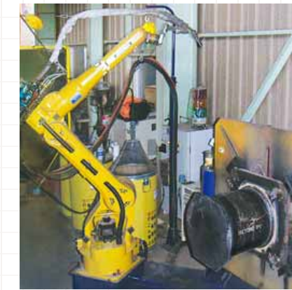
● Surface step sensing and burn through prevention function
