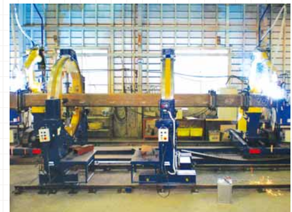
2-ARC welding joining HSS-column core
