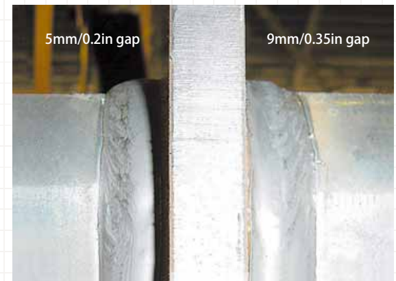
Example of effect on thin plate (effect on 2-ARC thin plate)
