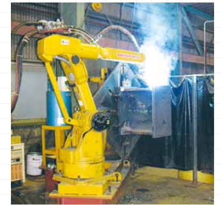
● Burn through prevention function (Example)
