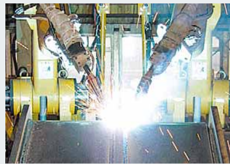
Central diaphragm is simultaneously welded.
